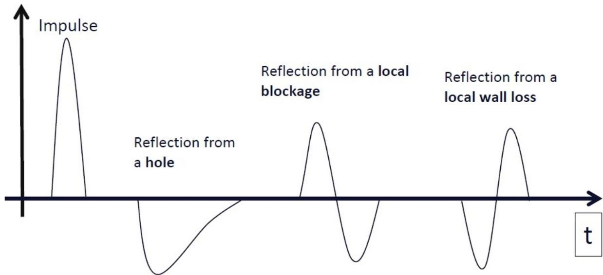
Figure 2: Theoretical signatures of most common defects
